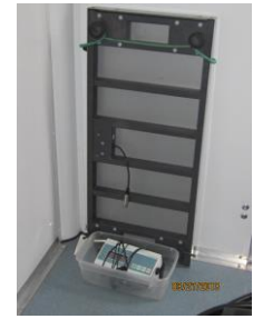
A veterinary scale travels with its’ feet out or upside-down, so the feet don’t hit a hard surface.
